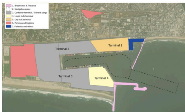
Figure 7: Port layout in current situation (left) and future situation (right) with planned development components
