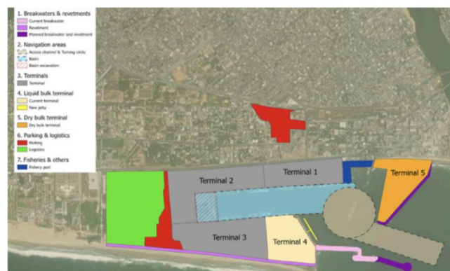
Figure 7: Port layout in current situation (left) and future situation (right) with planned development components
