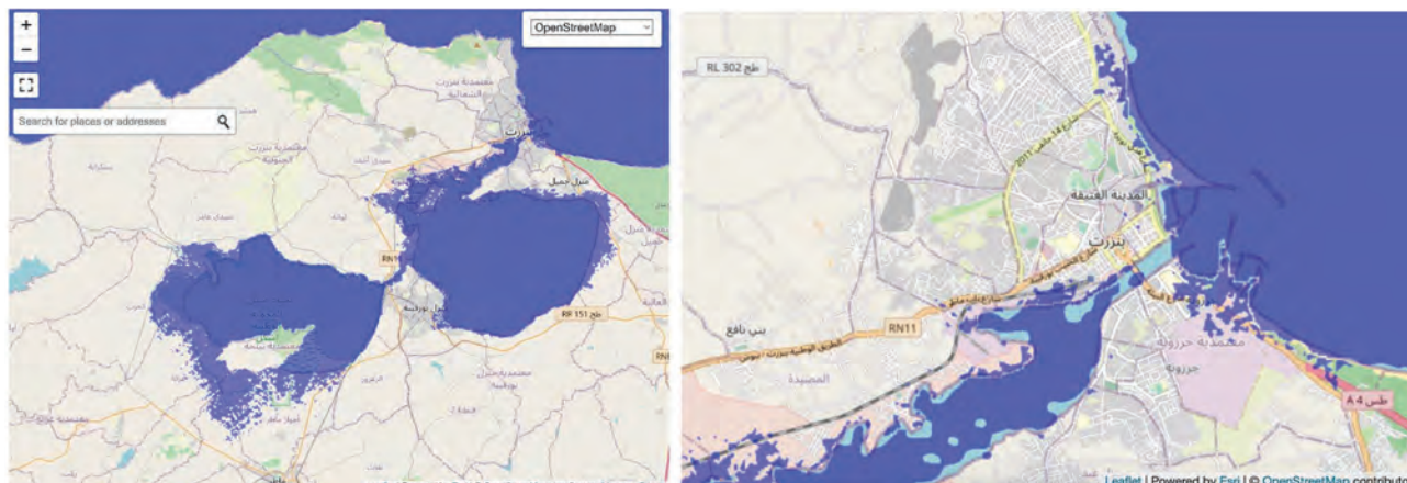
Figure 3. Areas Anticipated to be Submerged with Sea-Level Rise In Bizerte, Largely Limited to Areas around Lake Bizerte and Lake Ichkeul
