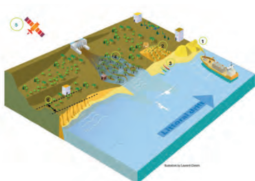
Figure 3. Soft Engineering, Coastal Planning, and Risk Management Solutions (left), and Hard Engineering Solutions (right)
