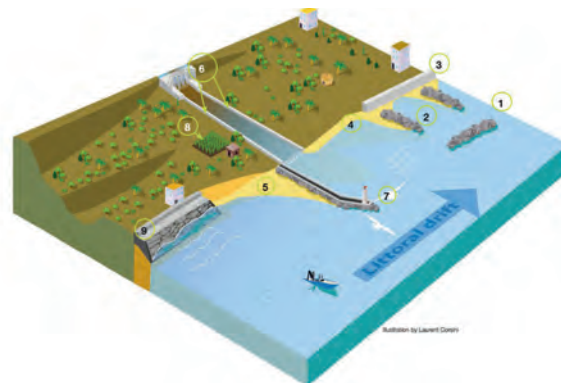
Figure 3. Soft Engineering, Coastal Planning, and Risk Management Solutions (left), and Hard Engineering Solutions (right)
