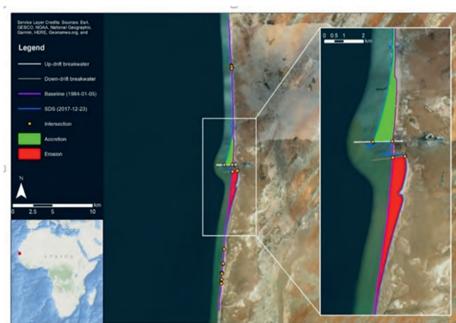
Figure 2. Beach Change Detected for the Port of Nouakchott (Mauritania) between Jan 1984 and Dec 2017
